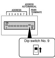
When setting the IP address on the digital video recorder
